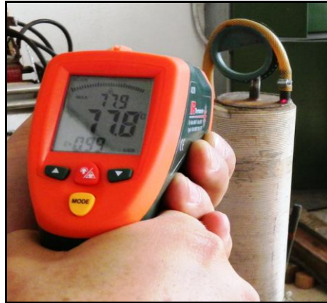
Fig. 4. Temperature measurement of the water coming out from the boiler.
